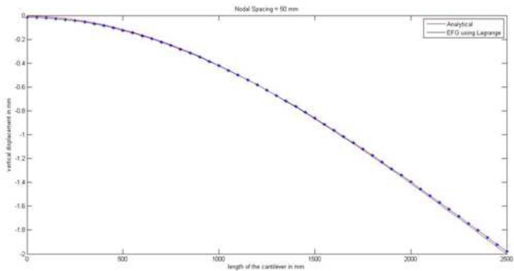
Figure 7: Comparison of Mfree Solution with Analytical Solution
