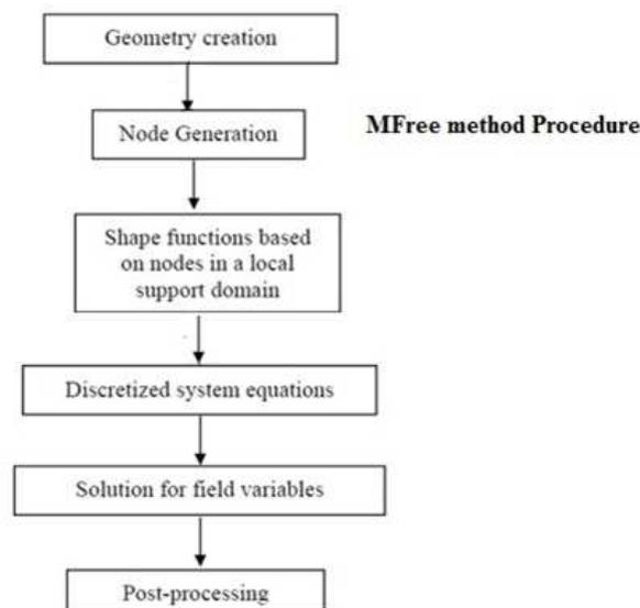
**Figure 1: Flow Chart of the MFree Method's Procedure**
