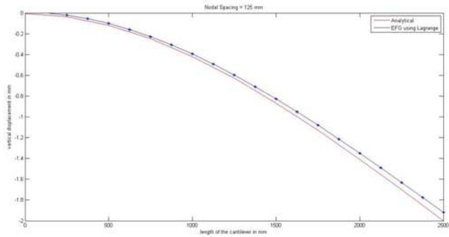
**Figure 4: Comparison of Mfree Solution with Analytical Solution**
