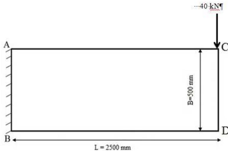
Figure 2: D Cantilever with Point Load at Free End
