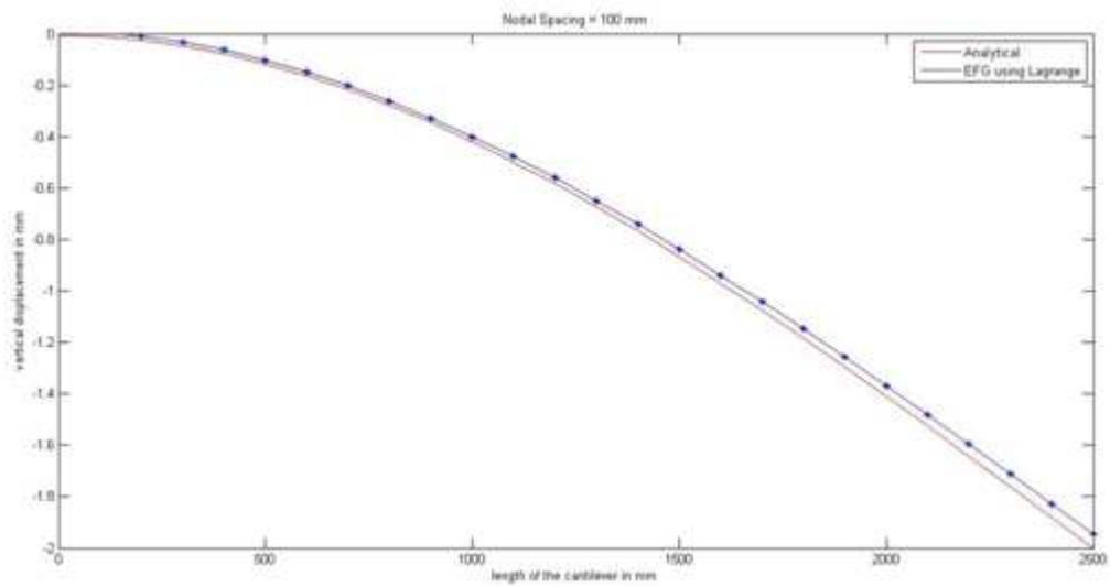
**Figure 5: Comparison of Mfree Solution with Analytical Solution**
