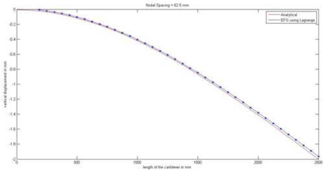
Figure 6: Comparison of Mfree Solution with Analytical Solution
