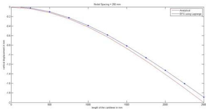
Figure 3: Comparison of Mfree Solution with Analytical Solution
